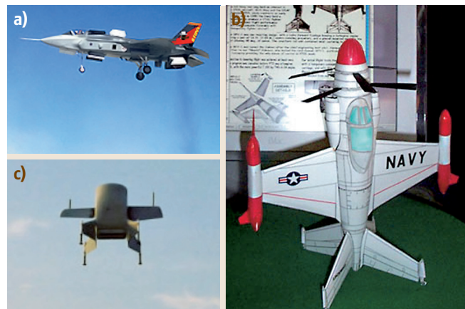
Fig. 44.9a-c Non-helicopter, hover-capable vehicles: (a) Joint Strike Fighter, (b) 1950s tailsitter aircraft and (c) Aurora Flight Sciences' Golden Eye 100
