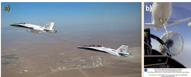
Fig. 44.14a,b Automatic airborne refueling. (a) Typical refueling configuration. (b) Camera view of refueling basket (Source: NASA Dryden Flight Research Center)
