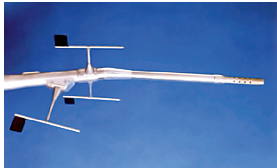
Fig. 44.11 Air data probe (Source: NASA Dryden Flight Research Center). The vanes are used to measure angle of attack and sideslip angle
