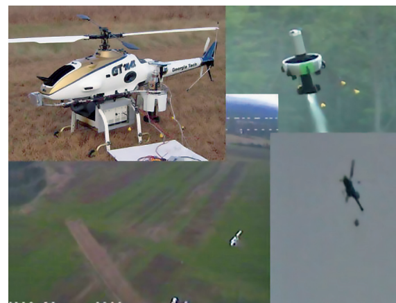
Fig. 44.15 Georgia Tech’s unmanned helicopter in a parent-child configuration. The child is a hover-capable ducted fan
